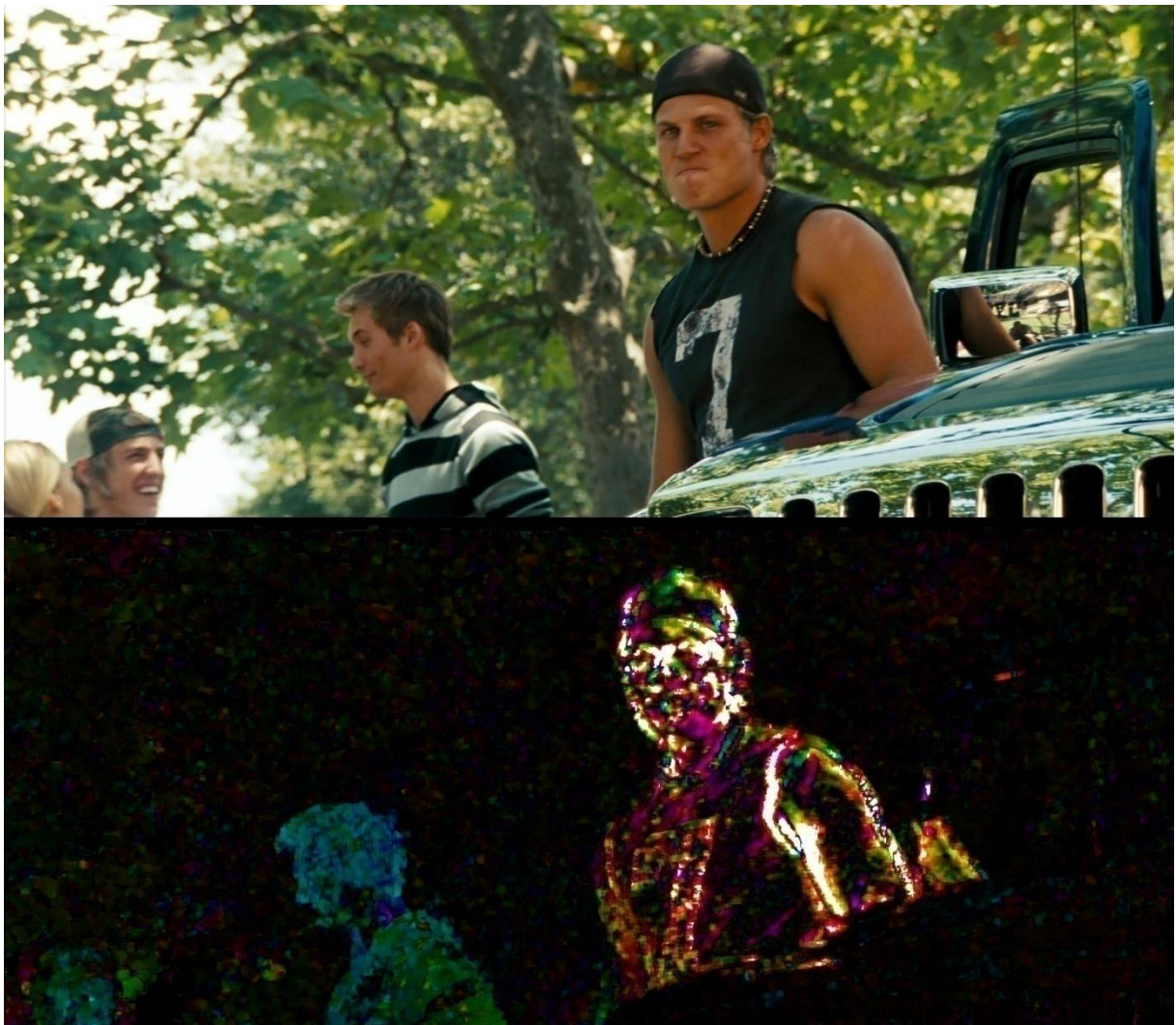
Figure 4.2. Screenshot of an image frame. The direction in which the pixels are moving can be determined by looking at the color scheme in figure 4.1. Pixels that are not moving are black.
